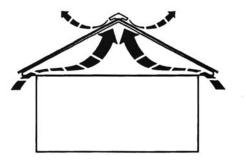
Ventilation requirements can range from 1 sq. ft. of ventilation for every 300 sq. ft. up to 1 sq. ft. of ventilation for every 150 sq. ft., according to the Asphalt Roofing Manufacturers' Association (ARMA) and the Canadian Asphalt Shingle Manufacturers' Association (CASMA). Ventilation requirements will vary depending on factors including the slope of the roof, and the type of roof.
